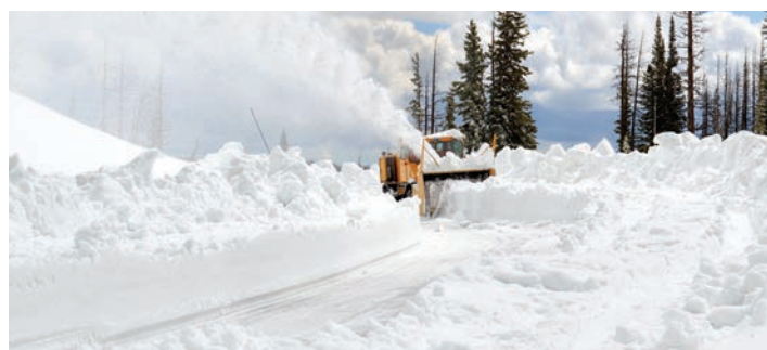
A rotary plow in District 1 clearing Snowy Range pass in late spring 2016.
